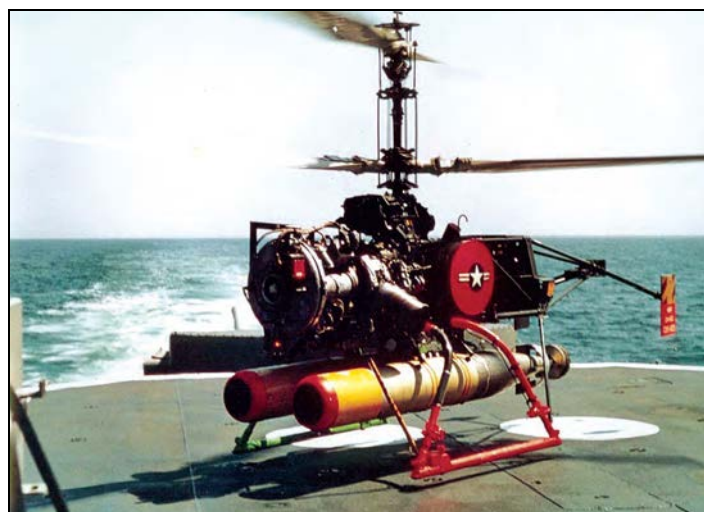
Figure 2: QH-50 DASH Testing aboard US Navy Destroyer.
